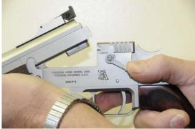
To close the action, hold the grip securely in your strong hand while pivoting the muzzle of the barrel upwards with your weak hand until the top slide is completely closed.
