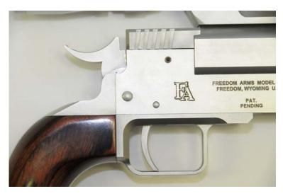
**AWARNING** If the hammer does not automatically move back to the safety position after firing (with the trigger released), unload your Model 2008 Single Shot Handgun and return it to Freedom Arms, Inc. to be inspected and repaired if necessary. Failure to do so may result in death, serious personal injury, and/or property damage.
