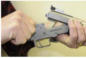
To open the action with the optional top slide lever, grasp the forend with your weak hand and the grip with your strong hand. Push the top slide lever down with the thumb of your strong hand while pivoting the muzzle end of the barrel down with your weak hand to open the action as shown in the photograph below.
