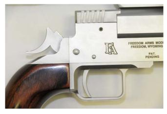
When the hammer is in the full cock position, pulling the trigger will cause the hammer to fall and strike the firing pin. When your Model 2008 Single Shot Handgun is fired, the upper front face of the hammer will momentarily be against the top slide before it automatically moves back to the safety position. Accordingly, when the trigger is released the hammer will be blocked from moving forward into the fired position.
