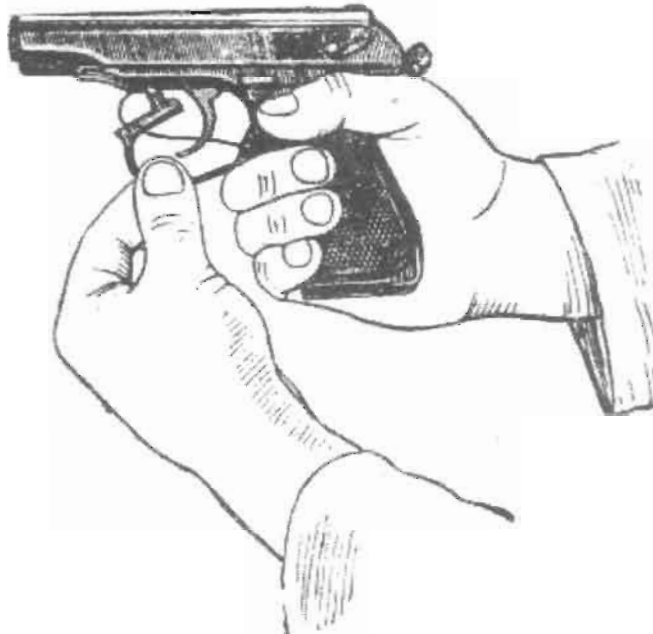
Picture 3.2 Pull Down Trigger Guard
