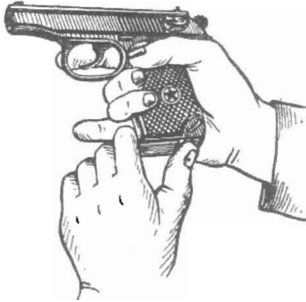
Picture 3.1 Removal of Magazine from the Frame
