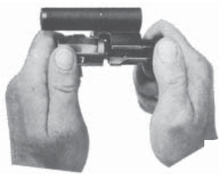
Fig. 37 Removing the bolt assembly components
