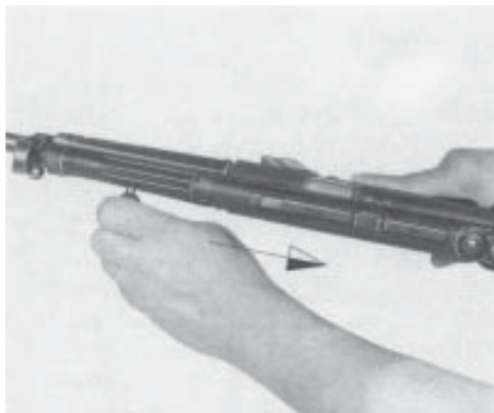
Fig. 31 Retracing the cocking lever Fig. 32 Releasing the cocking lever
