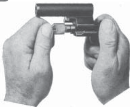
Fig. 38 Stripping the bolt assembly
