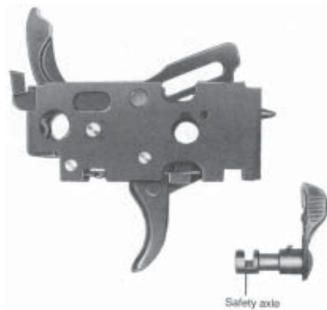
Fig. 16 Trigger mechanism and safety
